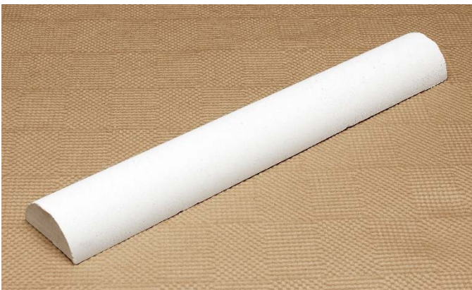
Silica/plaster mold for draping gecko.
