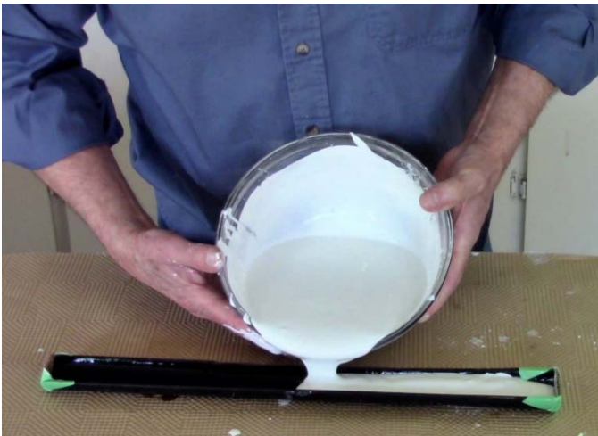
Making a mold by pouring silica/plaster compound into a strip of plastic plumbing pipe cut in half.
